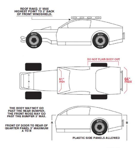
Rear quarter panel cannot be over 2" different left to right in total height. No flat or concaved roofs. Sail panels must be the same on both sides of the body and in the same location. (Plus or minus 2")
